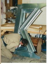
Twenty-three large brackets, 75 modillions and extensive cornice and frieze panels were fabricated and assembled in our shop.
